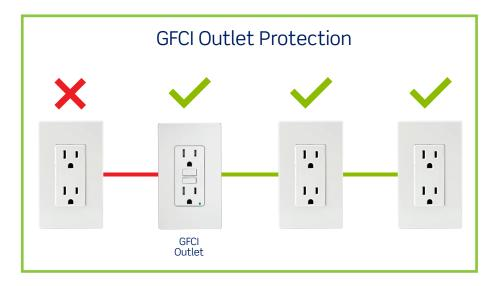
GFCIs protect against ground faults that can occur in the outlet face as well as in outlets wired downstream on the same circuit.
